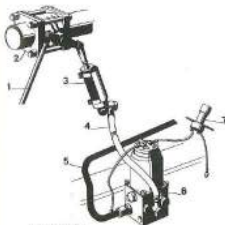
Exhaust brake 1 Spring link rod 2 Shutter housing 3 Compressed air cylinder 4 Line solenoid valve—compressed air cylinder 5 Line, compressed air reservoir—solenoid valve 6 Solenoid valve 7 Foot contact
