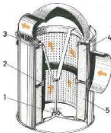
Air cleaner 1 Nut 2 Rubber ring 3 Clip 4 Cleaner element 5 Cleaner element
