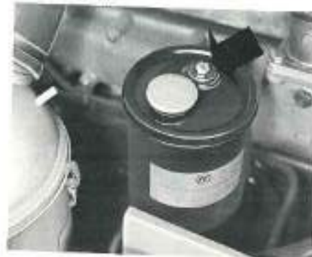
Removing oil filter
