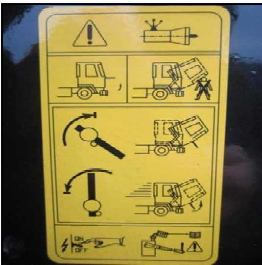
Fig 3-32 Cab tilting operations
