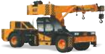
Mobile Cranes (9-80 Tonnes)
